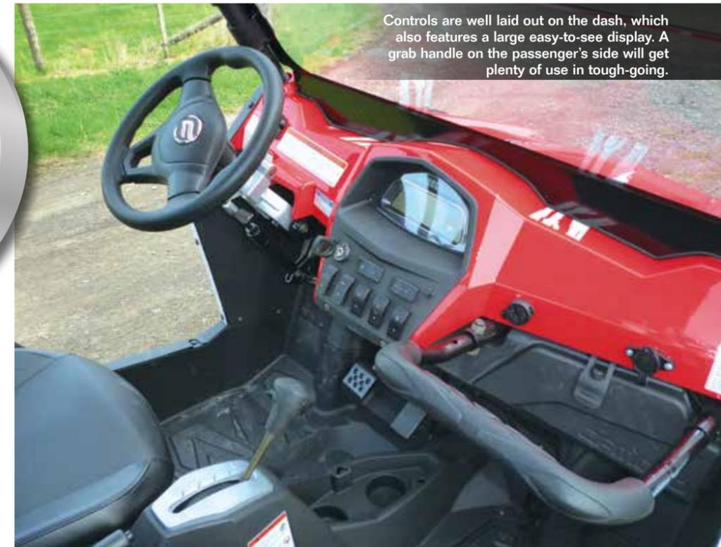
Controls are well laid out on the dash, which also features a large easy-to-see display. A grab handle on the passenger's side will get plenty of use in tough-going.
